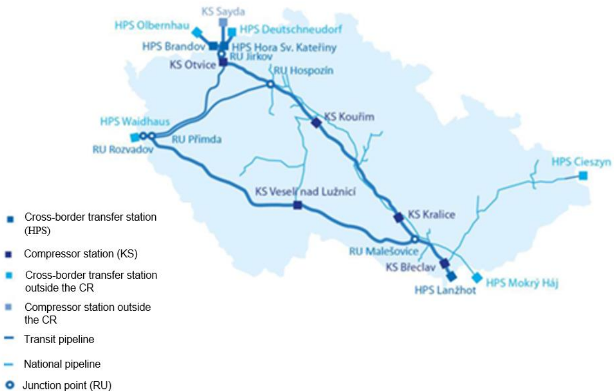
Figure 4 Structure of the transmission network
