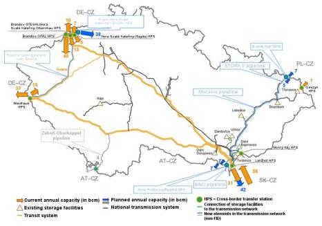
Figure 5 Map of entry and exit transmission capacities at cross-border transfer stations
