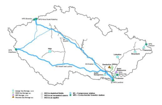
Figure 4 Map of storage facilities in the CR and their connection to the transmission network
