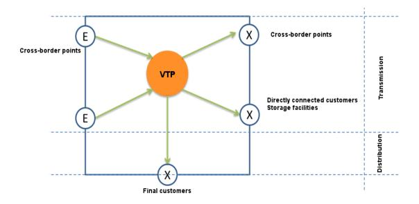
Figure 1 Schematic diagram of the Czech entry-exit system (source: ERO)
