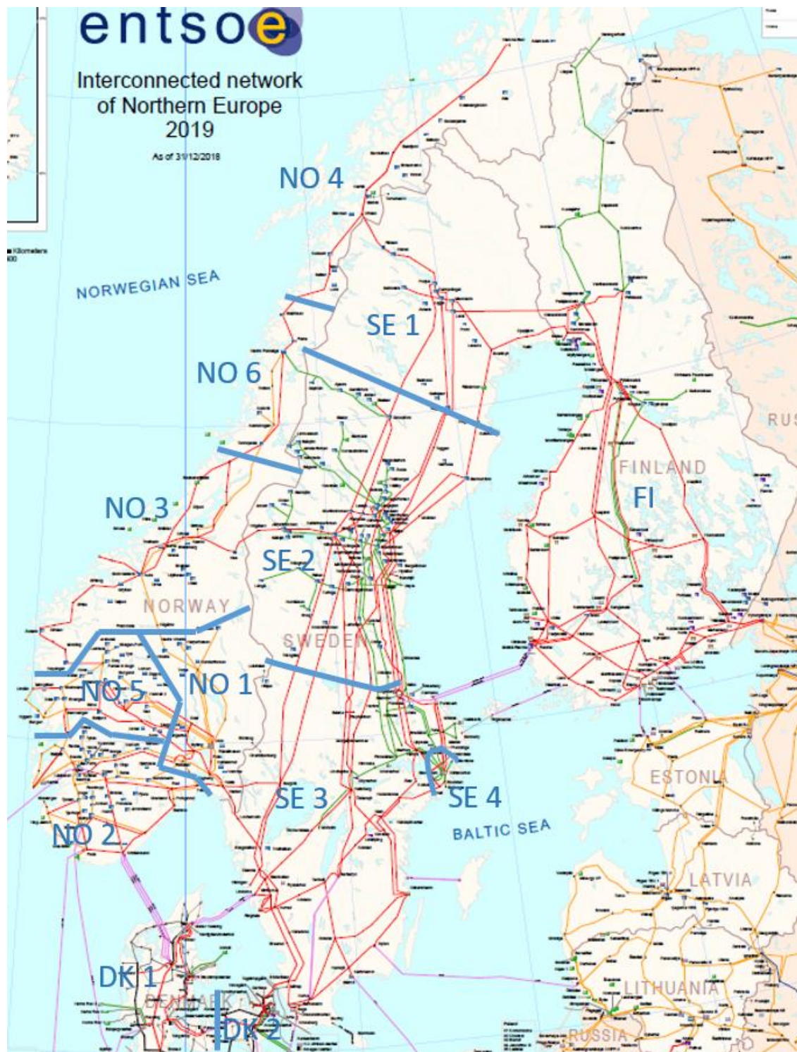
Figure B: Alternative configuration to be analysed for Sweden and Norway. In the proposed configuration regarding Sweden, a modified BZ SE3 is introduced in the Stockholm Metropolitan Area. The current BZ SE4 is expanded to include the remaining area of current BZ SE3. In Norway a split of NO4 is proposed, and a new BZ NO6 is introduced. For Denmark and Finland no alternative configuration will be assessed at this stage.
